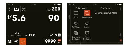
When Self-Timer, Interval, Exposure Bracketing, or Focus Bracketing is selected, the current configuration will be displayed to the right of the mode list.
