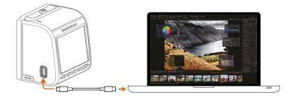
Connect the USB-C port on the camera to a computer using a USB-C cable of USB 2.0 or above. Users can control the camera remotely in Phocus, such as aperture adjustment or exposure time control.
