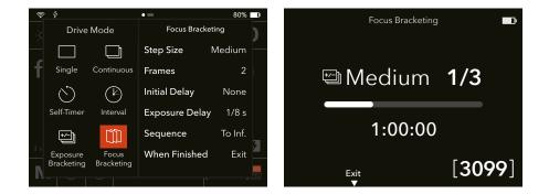
Step Size: The step of the focus position between frames. Refer to the following section for more information.
