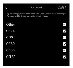
When using the CFV 100C with cameras other than the 907X, select the lenses here and the list of lenses for the lens data function in Browse mode will be limited to the selected models in this setting. Refer to the Image Browse section for more details about the lens data function.
